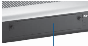
Easy access opening for HDD & CF
